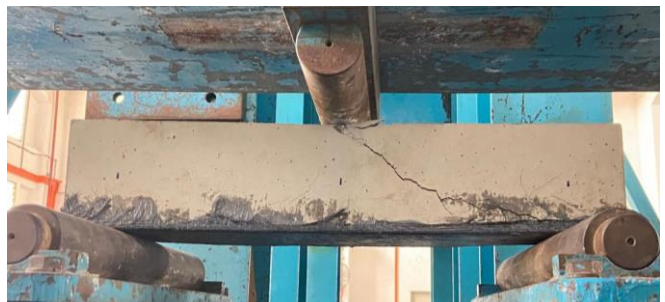
Figure 3 : Retrofitted RC beam with CFRP
