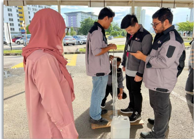
Students are conducting a pavement surface drainage experiment using an outflow meter
